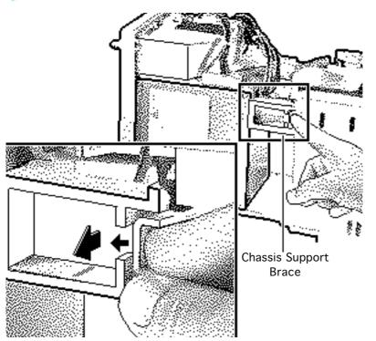
1 Remove the chassis support brace.
