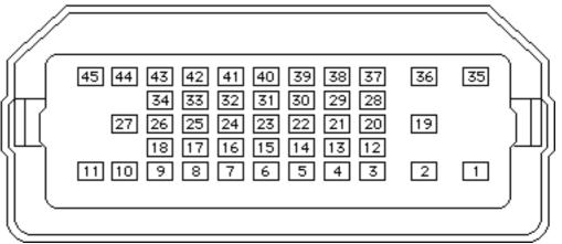
Figure: HDI-45 Connector on the Logic Board
