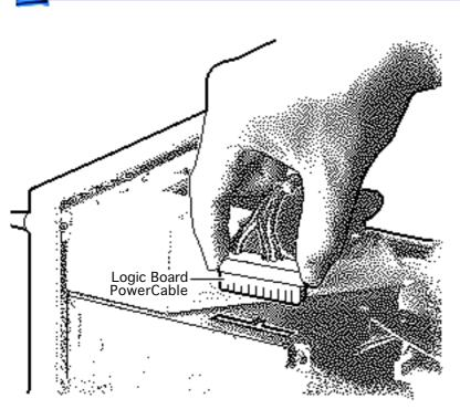
Disconnect the logic board power cable.
