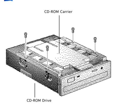
3 Attach the CD-ROM carrier to the CD-ROM drive with four Phillips screws.
