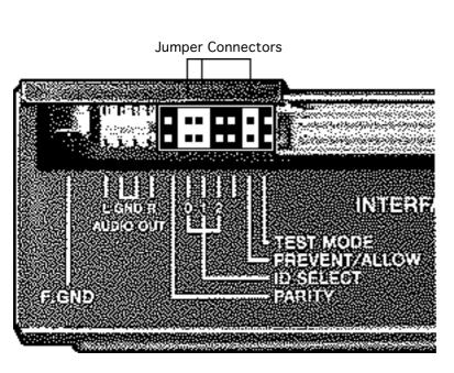
4 Verify that the three jumper connectors are installed as shown.
