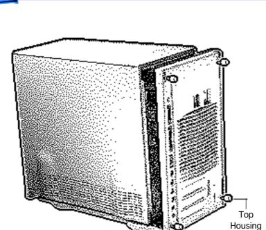
9 Move the top housing screws from the old unit to the new unit and reassemble the computer.
