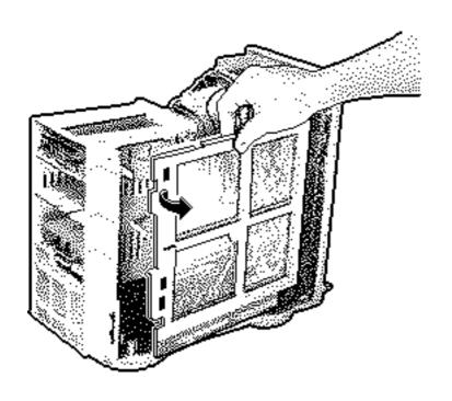
Pivot the front of the logic board out of the chassis.
