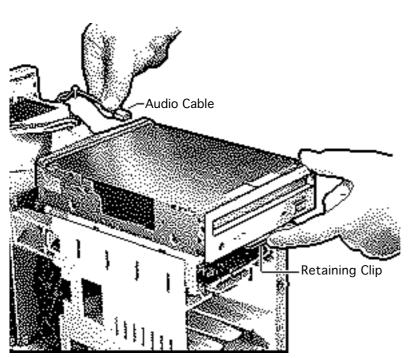
Disconnect the SCSI data cable, audio cable, and power cable from the back of the CD-ROM drive.
